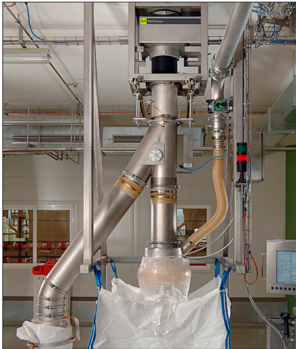
Installation example: IFS compliant metal detection directly before the filling of spice products into bigbags. (old version)
