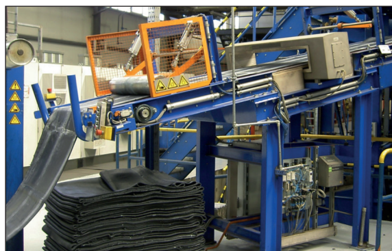
Installation example: GLS-R metal detector installed in a belt conveyor for the inspection of rubber sheets in the tyre industry (old version)
