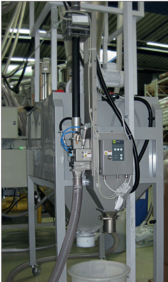
Installation example: Metal separator GF installed in a vertical pipeline (old version)
